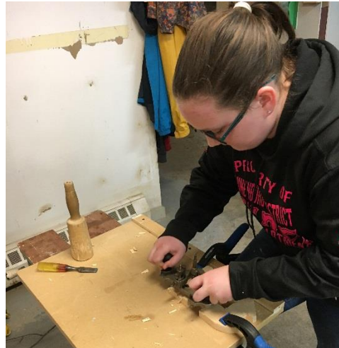
Nora using her Stanley No.71 router plane we purchased from Holley Jayne last fall.
